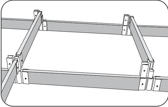
2) For the second level, place six 4-way bracketed timbers (FW) on top of the 1st level (see diagram 2), then add parallel-bracketed (PB) timbers as marked on diagram 4.
