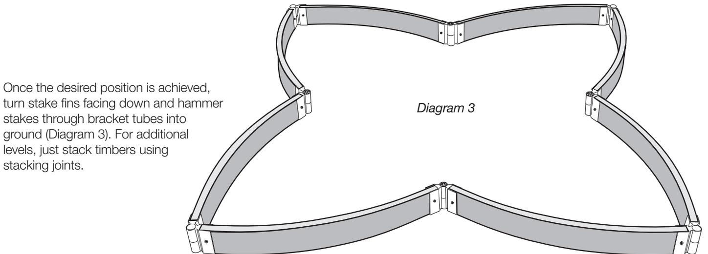
Once the desired position is achieved, turn stake fins facing down and hammer stakes through bracket tubes into ground (Diagram 3). For additional levels, just stack timbers using stacking joints.
